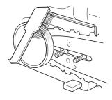
Regularly check that the brake band is at least 0.6 mm thick at its thinnest point.
